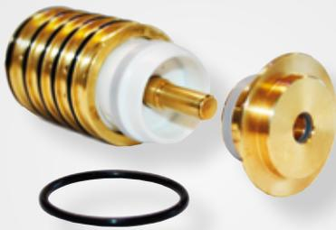
The TF series is equipped with a special, hybrid air valve comprising of a brass body and PET cylinder. The cylinder is made of a light material therefore it does not damage the air valve housing and the pump center body at high pressures.
