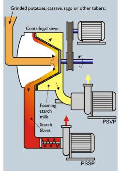
The PS Series of Stainless Steel AISI 316 Pumps has been designed specifically for use within starch production processes. Characterised by smooth internal finishes, optimal hydraulic performance as well as their unique and modular design with ample sealing choices, means these pumps are a perfect, onestop, solution for all duties affiliated with the different stages in starch production.
