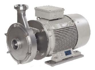
Specifically designed for the transfer of partially de-foamed Starch Milk to hydro-cyclones within the starch production process. The principle of design is based around high efficiency, low maintenance costs and ease of assembly and disassembly, such as back pull-out of the front cover / casing.
