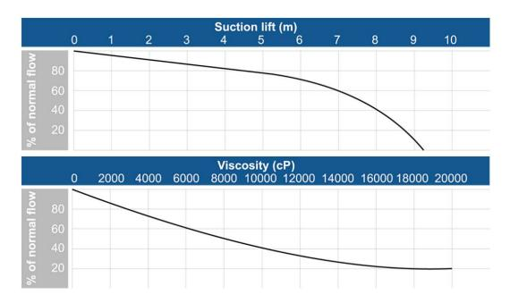
All performance charts are based on test done with water, therefore, if an application demanded a 4 m suction lift on a fluid that was approx. 3000 cPs, then potentially a larger pump which could produce 40% more capacity would be required.
