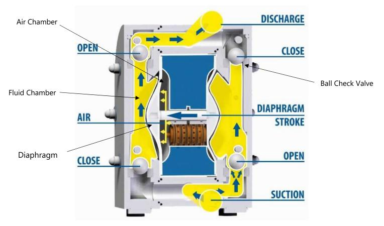
An Air Operated Diaphragm Pump is principally made up of 2 Liquid Chambers, 2 Air Chambers and 2 Diaphragms. The Liquid and Air Chambers are separated by a Flexible Diaphragm.
