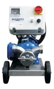
The INV BS Series is a simplified and more cost effective alternative to the INV series. It is characterised by featuring either the close coupled MINOR 40 or MAJOR 60 pump units fitted with forced ventilated motors onto a 2 wheel trolley system. All flow control is located on the control panel and dry run protection isn't featured. Speed adjustment range has been limited to 175 – 1400 rpm due to the absence of a gear box, as opposed to a minimum speed of 50 rpm capable with the INV series.
