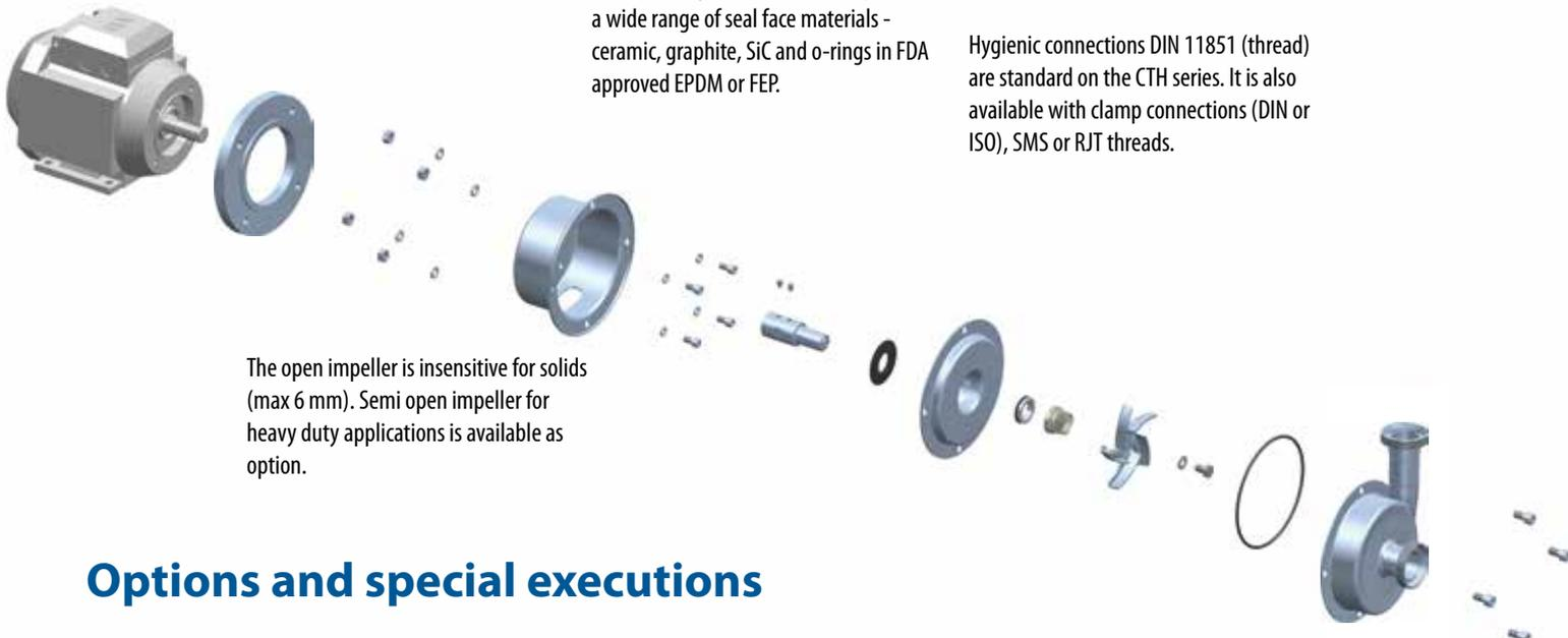
Standard single mechanical seal provides a wide range of seal face materials - ceramic, graphite, SiC and o-rings in FDA approved EPDM or FEP.
