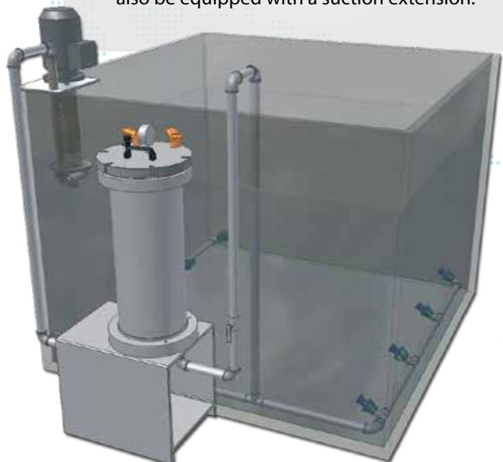
CTV is commonly installed in surface treatment baths, circulating through filter and further to nozzle ramps.
