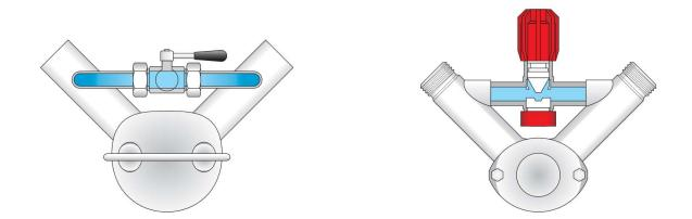
Manual and Spring Loaded By-Passes are available on all pumps can are ideal when the pump is being used with a discharge nozzle or there is the potential for Dead Head Operation.
