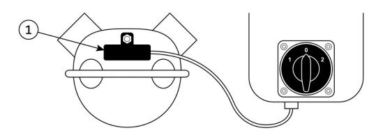
Dry Run Protection can be fitted to pump heads from MINOR sizes upwards. It is a temperature sensor which automatically stops the pump once it registers a temperature higher than 50°C within the pump head. For fluids being pumped higher than this temperature then sensors set at 70 & 90°C are available on request and need to be specified at order stage. Once the temperature in the pump head drops below the pre-set value the pump automatically starts back up.
