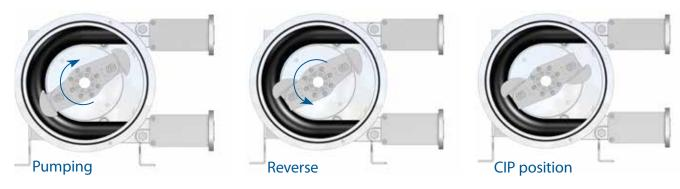
PT pumps are available in "CIP wheel" (Clean In Place) option. It allows users, by simply reversing the direction of rotation of the pump ( $\frac{1}{2}$  turn), to be able to retract the shoes automatically, in order to make the cleaning and sterilization operations, without any action on the pump. The client saves time and will keep the highest level of functionality in the process.
