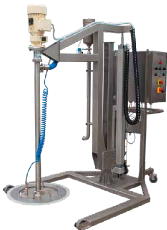
HVS Flexi system with a lip seal scraping lid for efficient single drums unloading.
