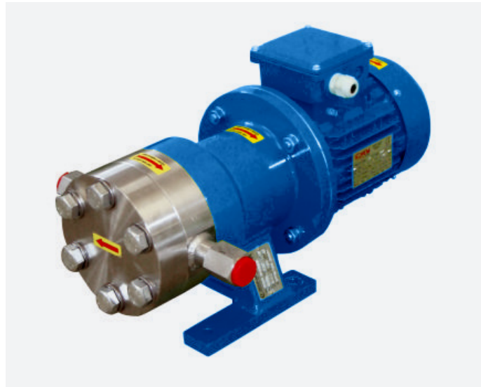
High Pressure Variation – Design pressure 710 Bar (10298 PSI) with hydrotest 1064 Bar (15433 PSI) –Material Superduplex SAF 2507.
