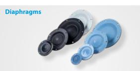
The composite design of Tapflo diaphragm makes it very durable even at higher operating pressures. Inside there is a reinforcement net and light metal core making it ideal for continuous heavy duty service. The face of the diaphragm is completely smooth so no metal parts come into contact with the pumped liquid and there is no leakage through it.
