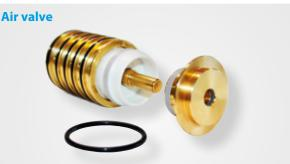
The TF series is equipped with a special, hybrid air valve comprising of a brass body and PET cylinder. The cylinder is made of a light material therefore it does not damage the air valve housing and the pump center body at high pressures.
