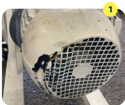
Damaged fan cowl
