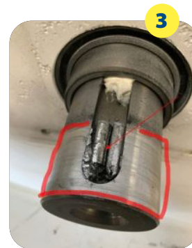
Damaged Hub Taper Lock
